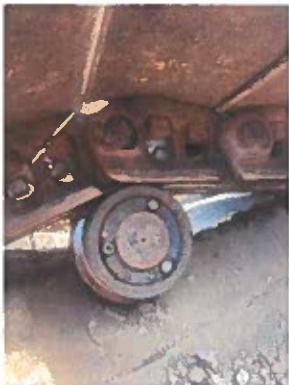
Image Comment(s): LH master pin walking out
