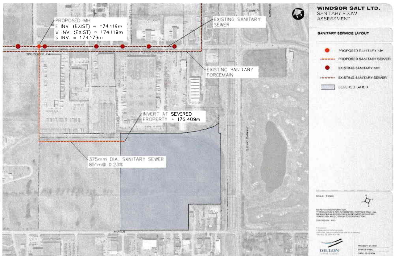
FIGURE 2: SANITARY SERVICE LAYOUT DILLON CONSULTING LIMITED www.dillon.ca
