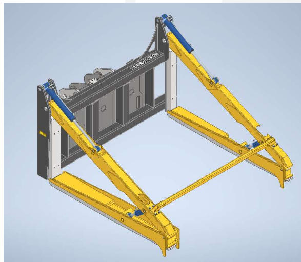
Figure 1: Pipe Handler (1-2393) and Fusion Coupler (1-2923) lifting attachment assemblies.
