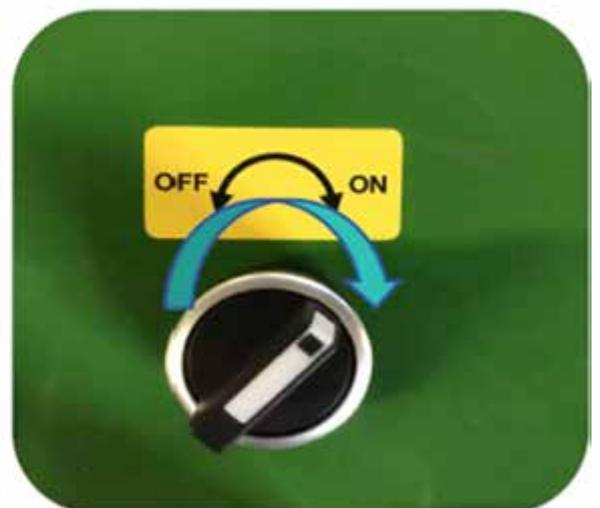
Paso 3, Active el interruptor del control Remoto ON.
