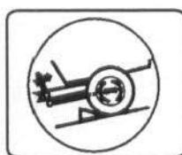
When parking use prop stand, handbrake and wheel chocks.
