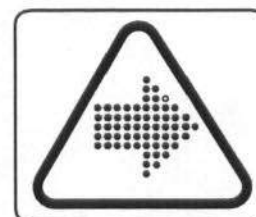
Air/gas flow or Air discharge.
