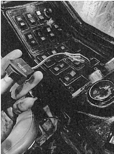
Dither switch replaced with new.
