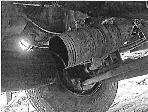
All the flex pipe is broke on Exhaust
