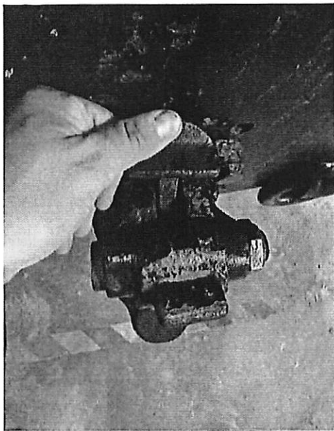
Broken safety latch ears on Pintle hitch
