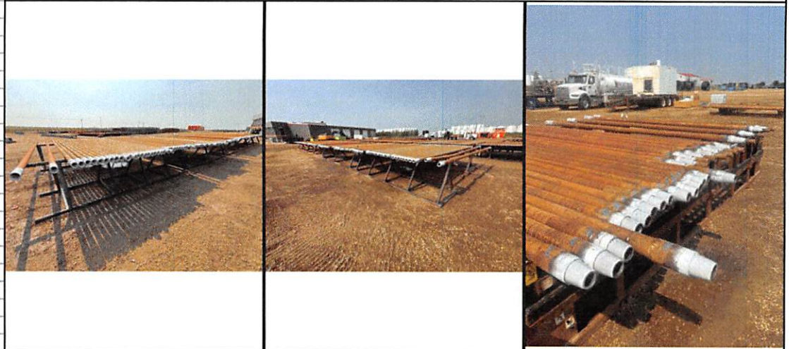
TYPICAL BORE PIPE
