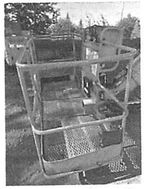
P9.4: Bent top rail (suitable for service)
