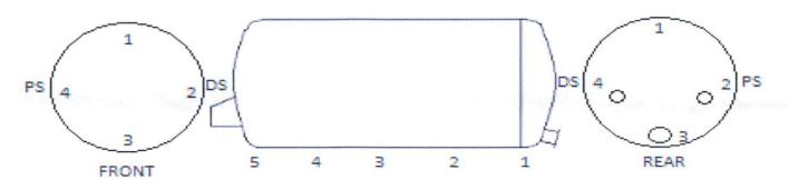
Measurements taken every 6' starting at rear of tank at numbered intervals in 4 positions. Front and rear measurements as numbered.
