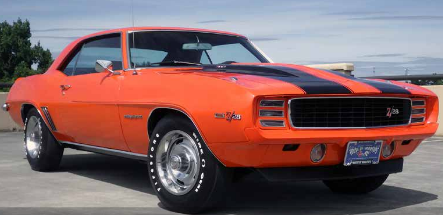
1969 Chevrolet Camaro Z/28 Coupe 302/290hp DZ hi-perf V8 engine with dual 4 crossram package / M21 4-speed manual transmission
