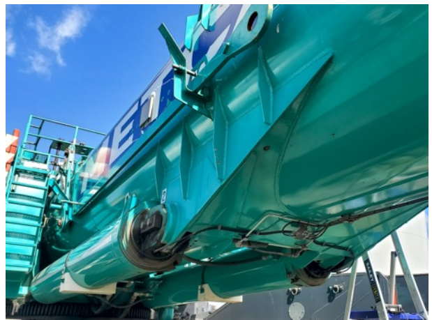
Luffing cylinder weld & mount
