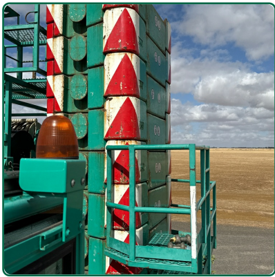
Counterweight Hazard Striping
