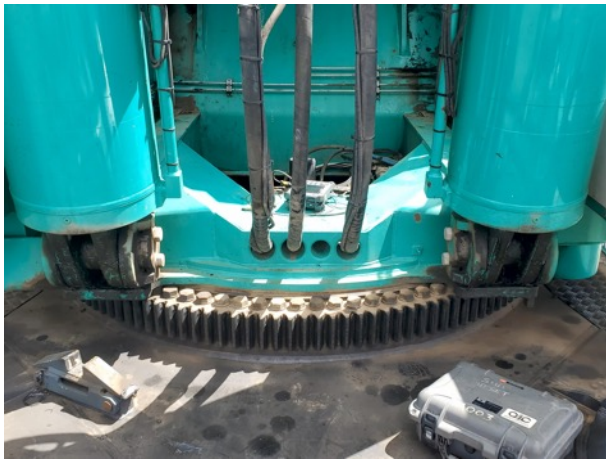
Luffing cylinder weld & mount
