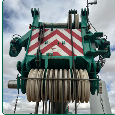
Head Sheaves and bearings
