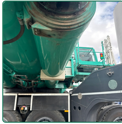
Boom Lift Cylinders
