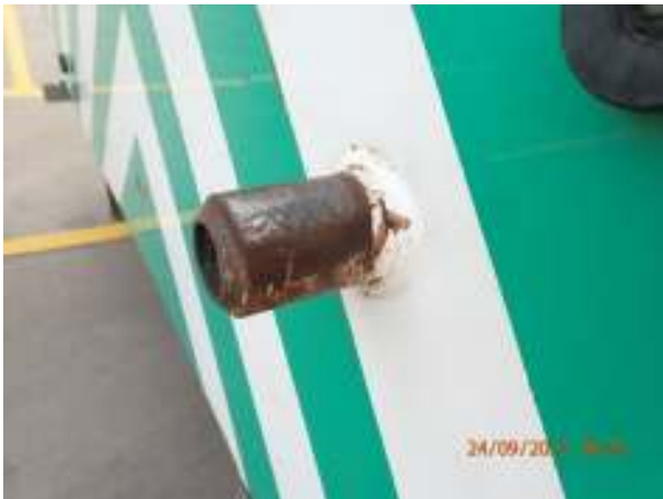
Photo 17: Front counterweight lug
