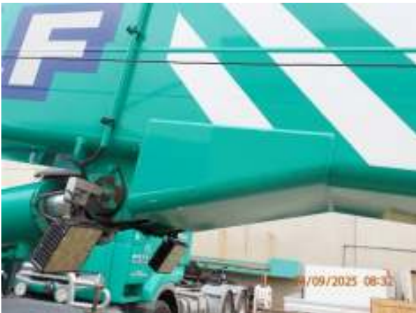
Photo 5: Upper luffing cylinder mount
