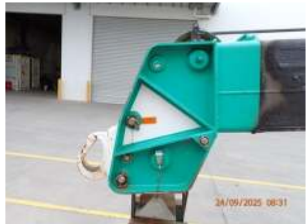
Photo 14: Boom tip and rhino hook
