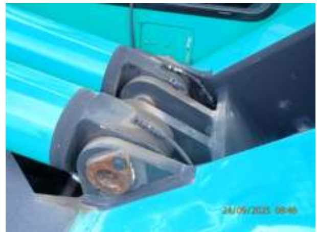
Photo 4: Lower luffing cylinder mount
