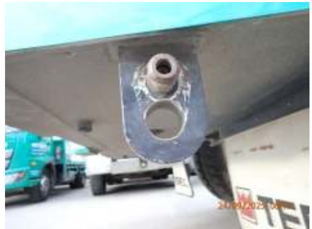
Photo 18: Rear counterweight lug
