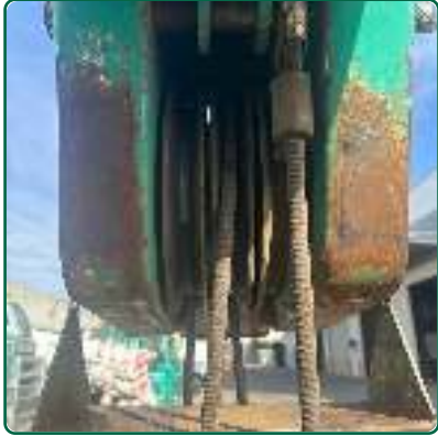
Head Sheaves and bearings
