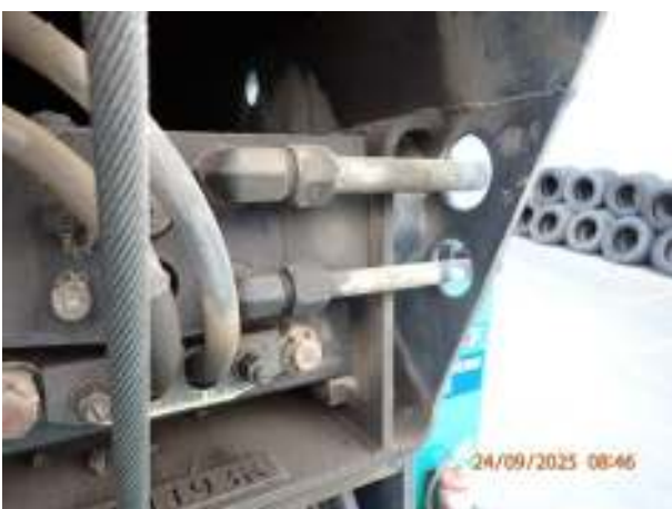
Photo 9: Boom telescopic cylinder mount
