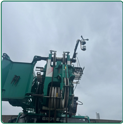
Idler Sheave and Bearing
