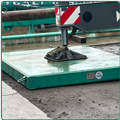
Vertical Outrigger Cylinders
