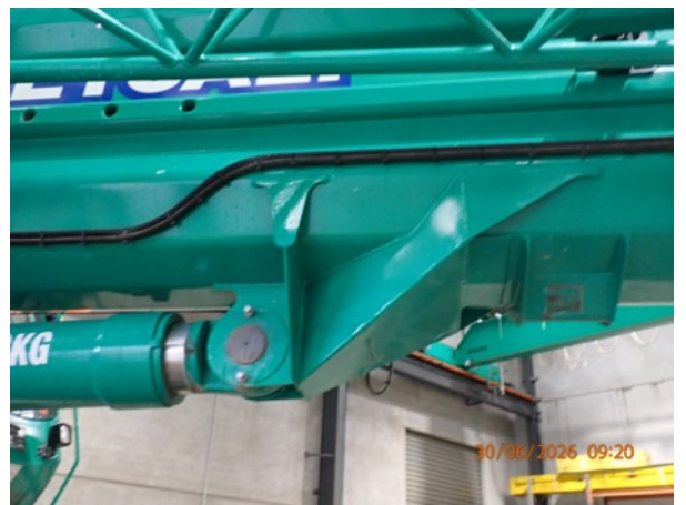
Photo 14: Upper luffing cylinder mount
