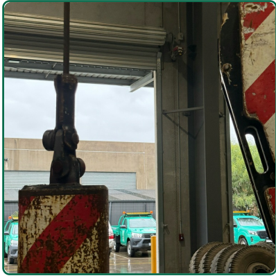
Correct Assembly and Connection of Auxiliary Hoist Rope Anchor
