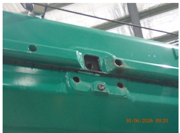
Photo 20: Boom pinning hole
