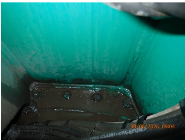
Photo 7: Inner slew bolts
