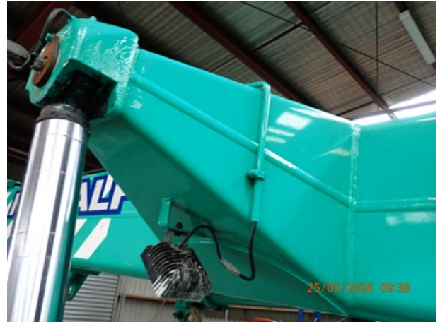
Photo 6: Upper luffing cylinder mount
