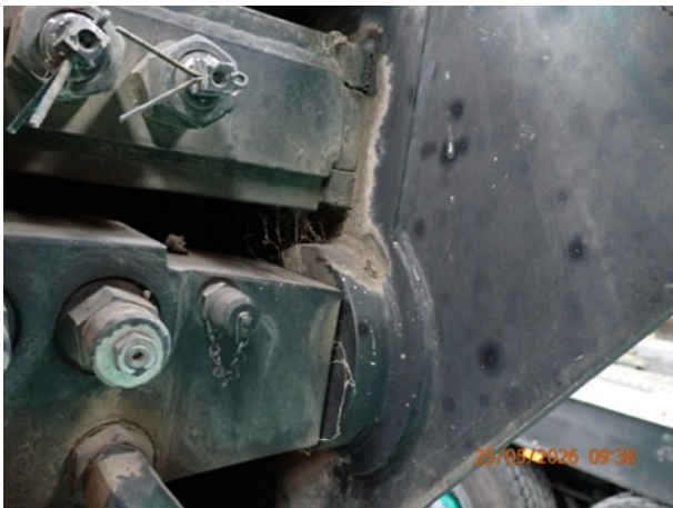
Photo 7: Telescoping cylinder & sheave mount
