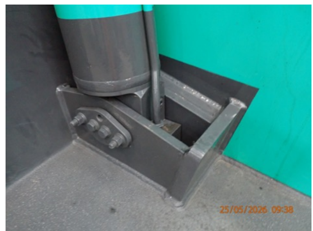
Photo 4: Lower luffing cylinder weld & mount
