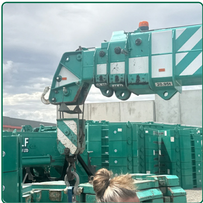
Boom Hazard Striping
