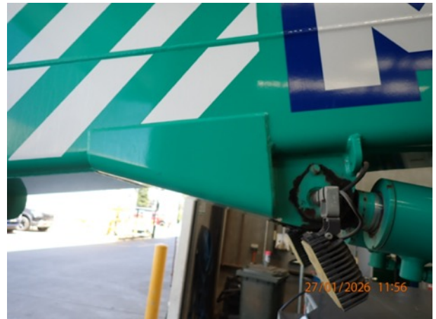
Photo 6: Upper luffing cylinder mount
