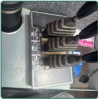
Control Levers - Clearly Marked
