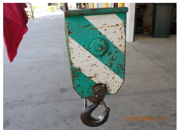
Photo 22: Hook & sheave block
