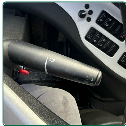
Transmission Retarder Working satisfactory at the time of inspection
