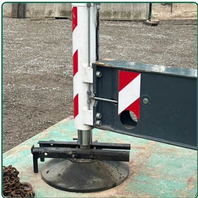
Outrigger Hazard Striping
