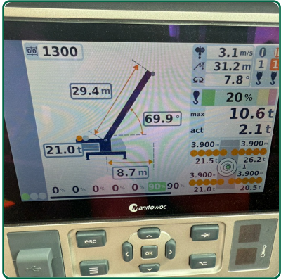
Line Pull Test
