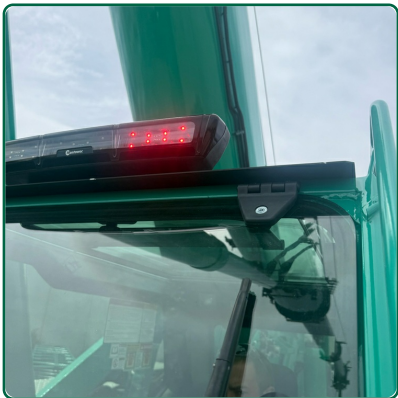
RCI Warning Lights and Alarms
