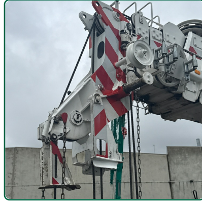
Boom Hazard Striping
