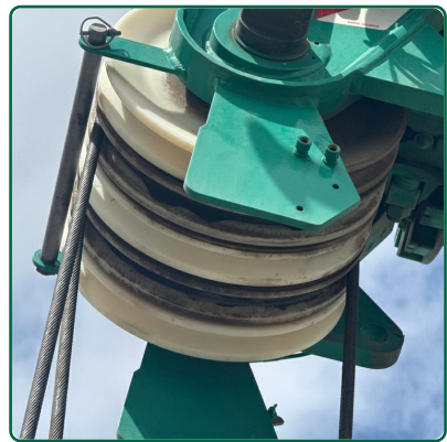
Head Sheaves and bearings
