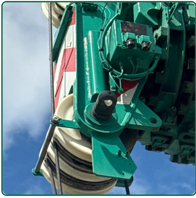
Boom Hazard Striping
