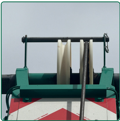
Idler Sheave and Bearing
