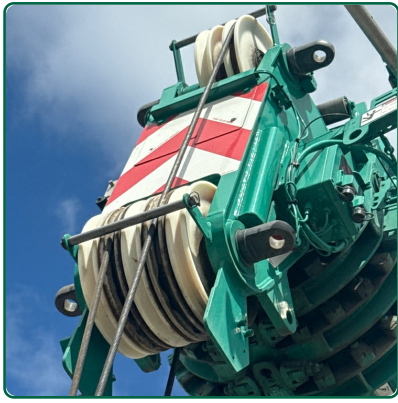
Sheaves and Bearings
