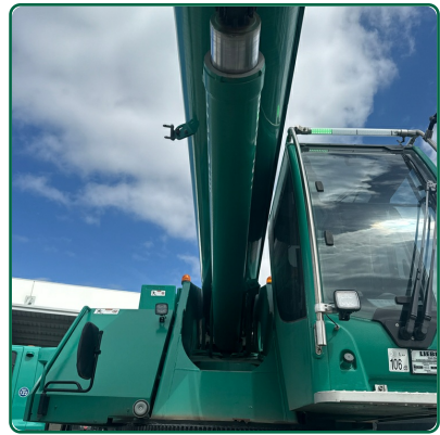
Boom Lift Cylinders
