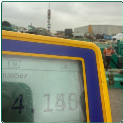
Load 4150 kg + hook block and rigging motion cut
