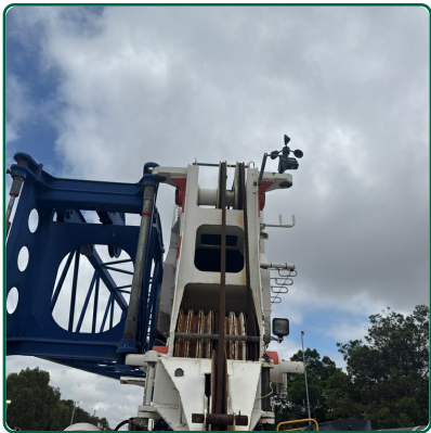
Idler Sheave and Bearing
