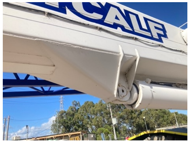
Photo 14: Upper luffing cylinder mount
