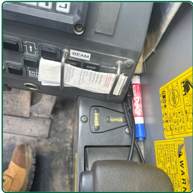
Crane Level Indicator
