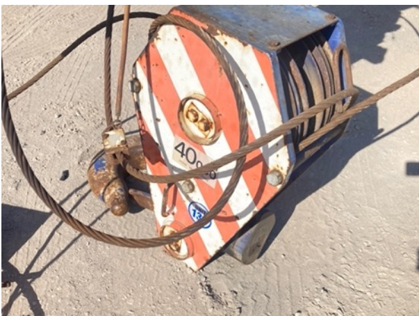
Photo 25: 40t hook & sheave block
