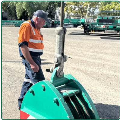
Main Hoist Rope Socket and Pins
