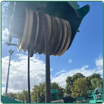
Head Sheaves and bearings
