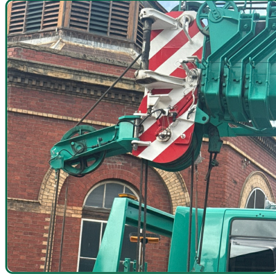
Boom Hazard Striping
