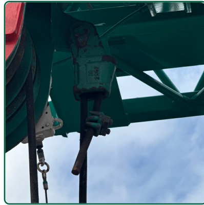
Main Hoist Rope Socket and Pins
