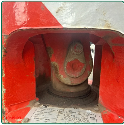
Correct Assembly and Connection of Auxiliary Hoist Rope Socket
