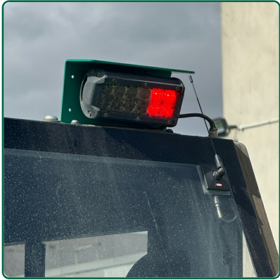
Overload Warning Lights and Alarms
