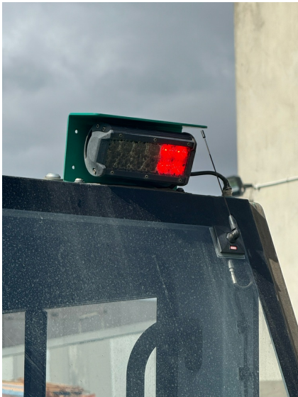
Overload Warning Lights and Alarms
