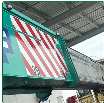
Boom Hazard Striping
