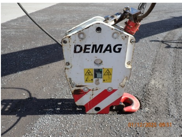
Photo 27: Hook & sheave block
