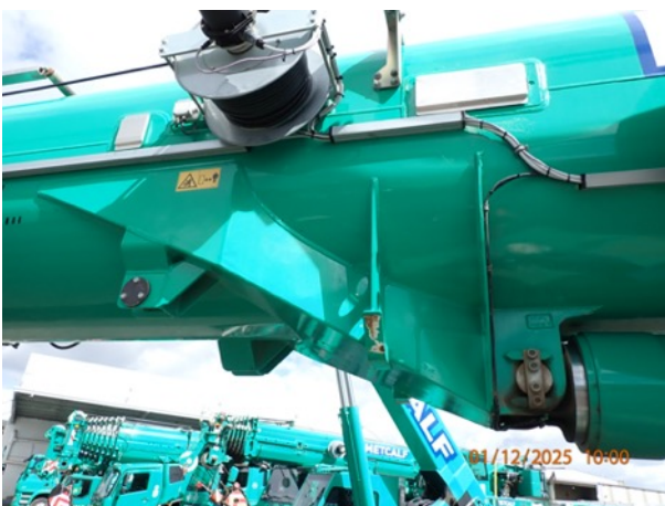
Photo 15: Upper luffing cylinder mount
