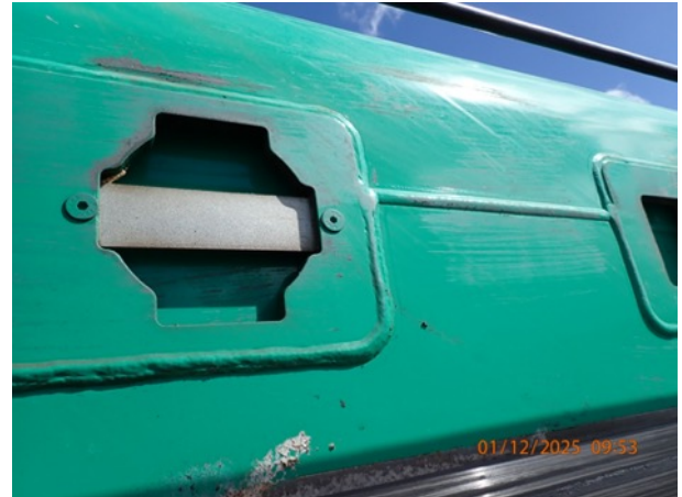
Photo 12: Boom pinning hole welds
