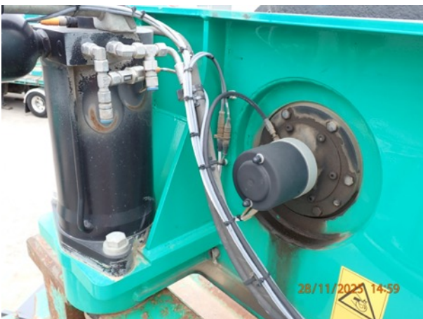
Photo 9: Winch & counterweight mounts
