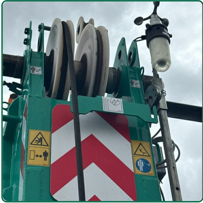
Idler Sheave and Bearing
