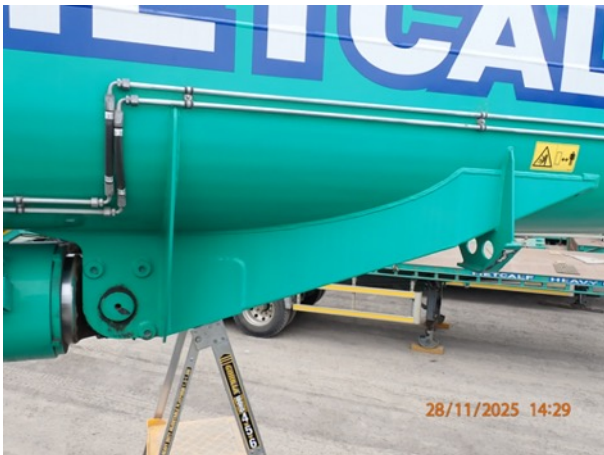
Photo 15: Upper luffing cylinder mount
