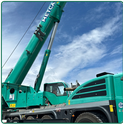
Boom Lift Cylinders
