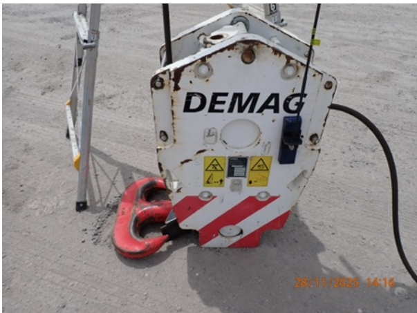
Photo 23: Hook & sheave block
