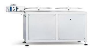
自动接封边条装置:采用红外探头检测,可实现两卷封边条, 自动拼接,实现不停机连续生产。 Automatically connect edge banding device: Using infrared probe detection, two rolls of edge strips can be automatically spliced to achieve continuous production without stopping the machine.
