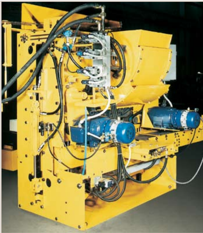
Valves are conveniently located for adjustment and maintenance. Vibrator motors are shown with optional Bescostop brakes.
