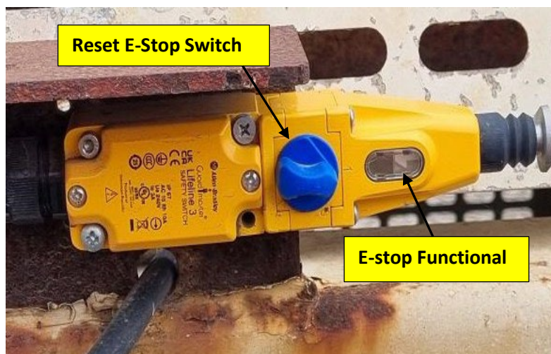
Lanyard (pull wire) type Emergency stop switch.
