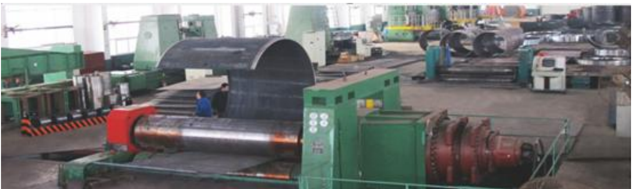
China biggest rolling machine for Max. 120mm thick steel
