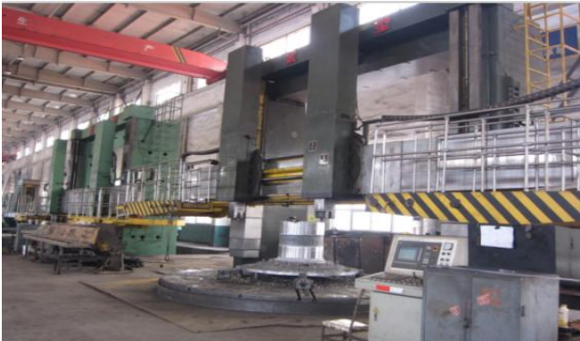
Heavy vertical lathe group with Max. Dia. 6m
