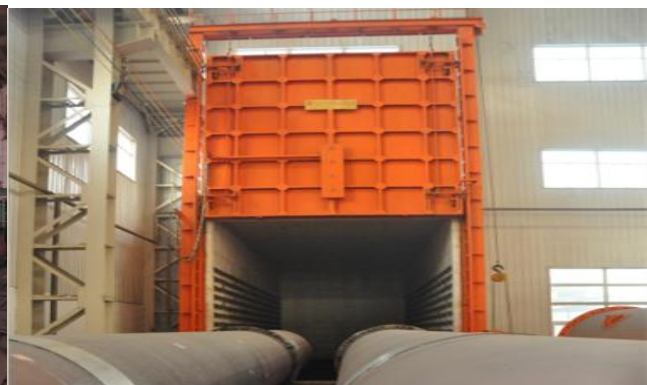
6*6*16.5m Automatic electric-heating annealing furnace
