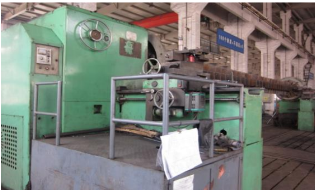
Heavy lathe for shell co-axiality (Max.Dia. 5m*26m )
